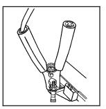
The remote positive (+) terminal is located under the engine compartment fuse block cover, and is marked with a plus (+) symbol on the cover. To access the terminal, remove the fuse block cover.
